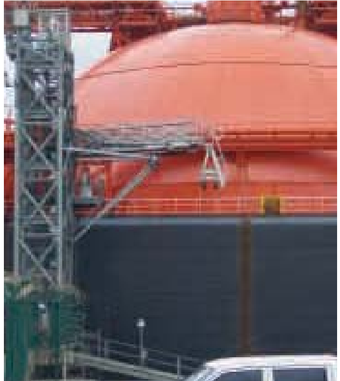
Tower gauging system
