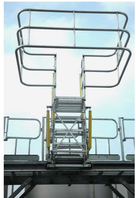
Folding Stairs are positioned next to chosen gate and then lowered on to the tanker. Picture shows a large 3-rail cage in aluminium.
