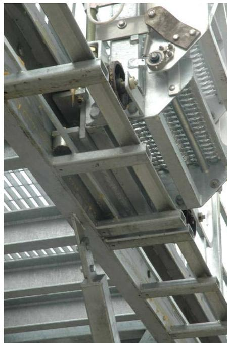
Unique track has wheel guides and hand-rail/gate system built-in
